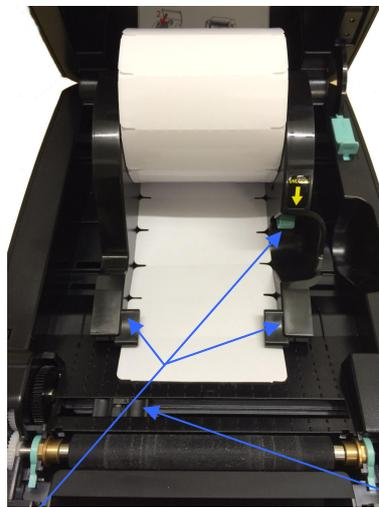
Adjust guides and install tape as above
