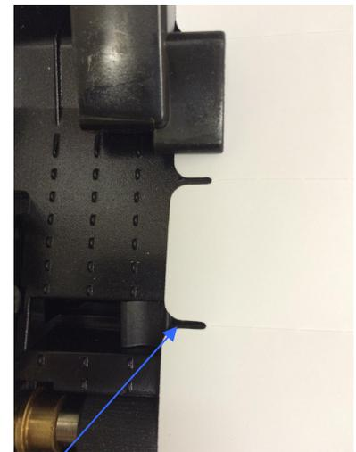
When using die cut tape ensure the sensor is located correctly to the tape cut-out
