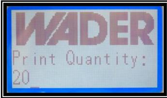
This particular label is made up of four lines only so now the screen prompts the user for a quantity of labels to print. For this example we have entered a quantity of **20**. Press the Return key and the printer will print the entered label 20 times. Once printing has finished the screen displays the print quantity in-case the user requires more of the same label (*different quantities may be entered*).
