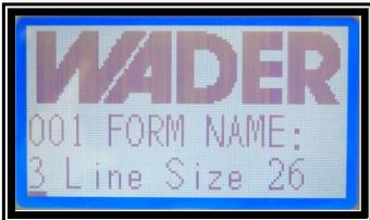
Stored label layouts are listed in alphabetical order, labels that have a numerical digit are listed first. Either press the arrow keys to scroll through the labels or press the first letter of the label layout name required to jump to that label.
