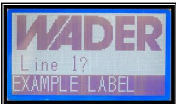
The Laundryprint will remember the label text entered. To leave the line as it is simply press the Return Key or type new text to replace it followed by the Return key. Repeat the processes for the remainder of the label as described previously.
