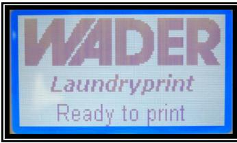
This is the Laundryprint main screen and is normally displayed if the system is not in keyboard mode.
