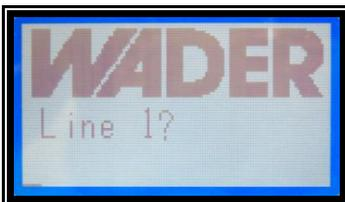
The screen will now display the first line of the label. The screen prompt for this particular label is "Line 1?" but this can vary in different label layouts.
