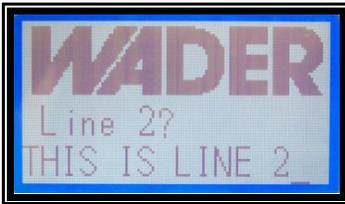
We are now prompted to enter text for line 2 of the label. For this line we have entered **THIS IS LINE 2** again after entering the required text press the Return key to precede to line 3 of the label.
